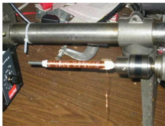
Small Drill press turned into a Coil Winder
